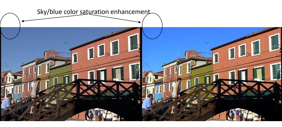
• The left side is represent the input frame to the contrast/color algorithm, the right side show the output. Minimum change to the skin-tones in the contrast and color processing.
