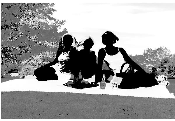
• Results from Blue/Sky detection algorithm. White indicates a Blue/Sky pixel. This information is used in the dynamic contrast algorithm and the color saturation enhancement algorithm.
