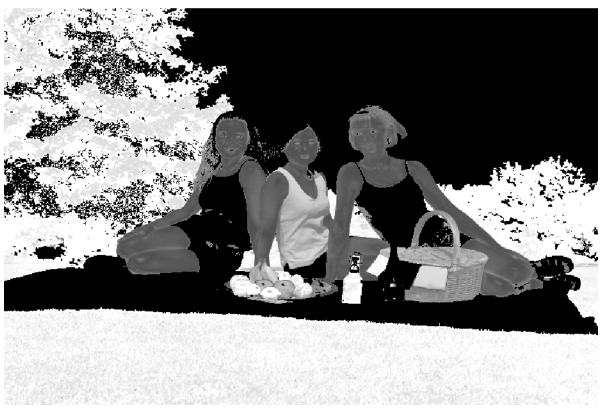
• Results from Green/Grass detection algorithm. White indicates a green/grass pixel. This information is used in the dynamic contrast algorithm and the color saturation enhancement algorithm.
